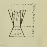
The stack of 13.75 in. diameter was not shortened.
